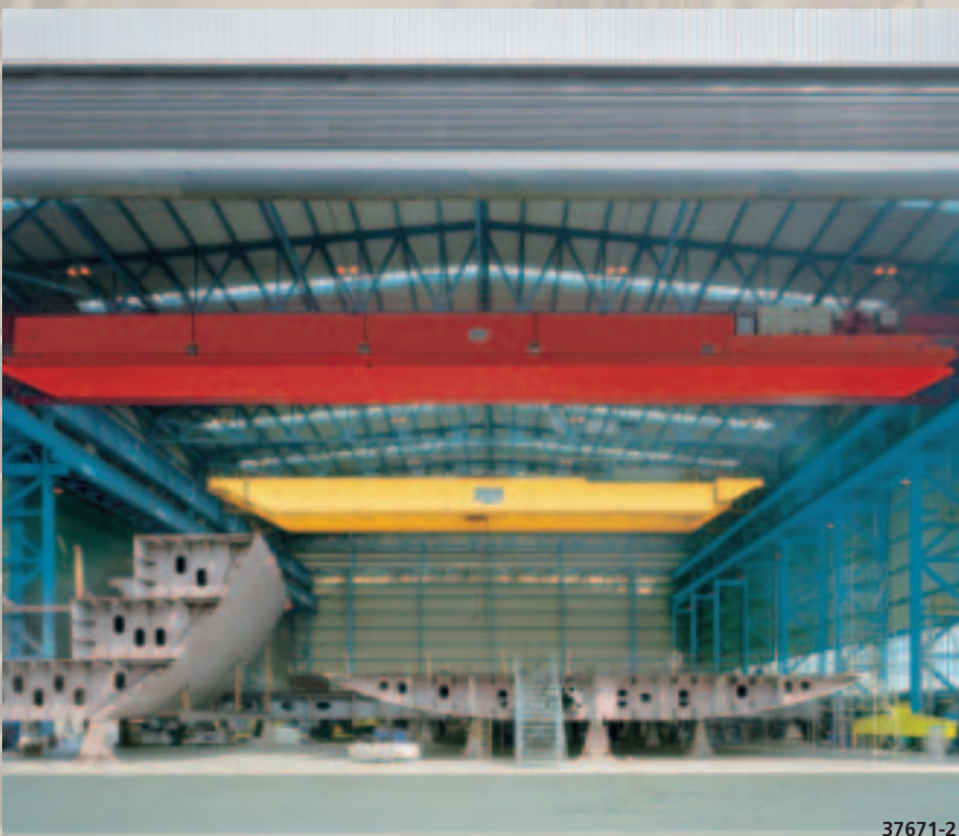
Changing load situations Double-girder open-winch cranes operating in a shipyard for the fabrication of ship sections.
